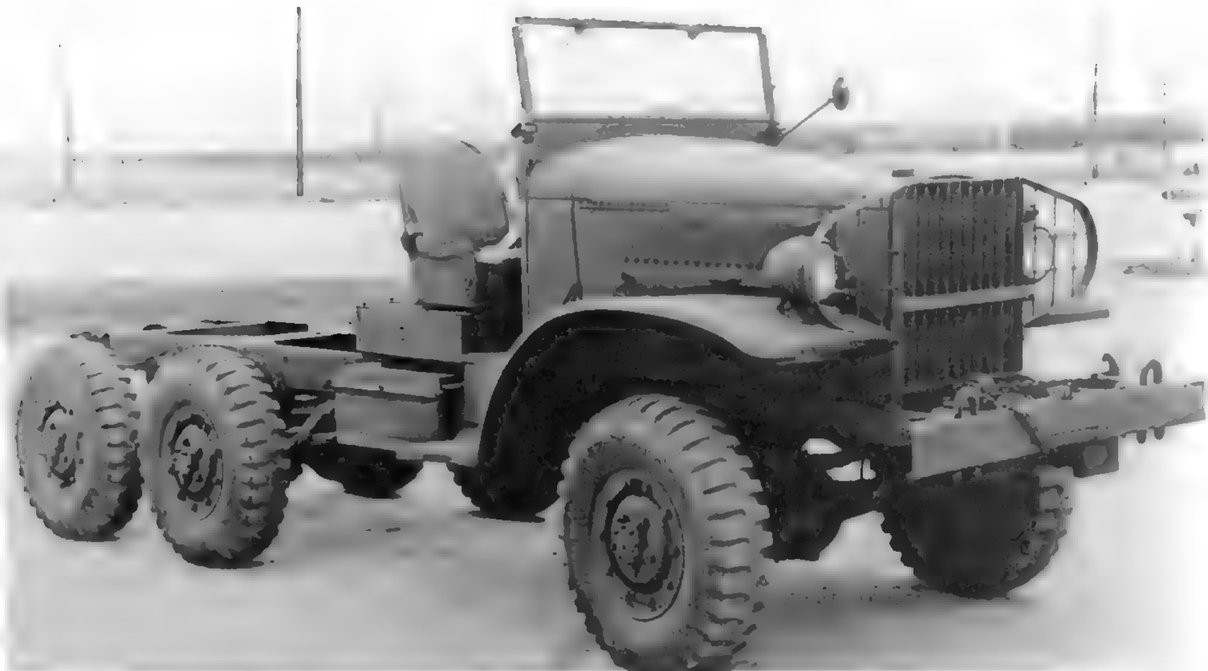
This M-3-6 was photographed during testing without its bed. The rugged business-like appearance is typical of International military trucks. (Photo courtesy of the Patton Museum)
